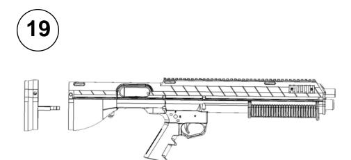
At this point reinstall the rear end cap making sure the detents lock in place. Your conversion is now complete. (conduct another function test).
