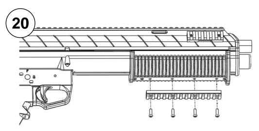
To install the accessory forearm rail (49) placed the unit upside down, align the four holes in the accessory rail with the four inserts in the forearm and install screws (12).
