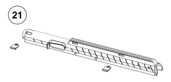
Your kit also comes with 2 sling attachment points. These can be inserted from right or left side depending on which side you want your sling on. The slots in the front and rear of the upper are for 2 point sling, the slot in the center is for a single point sling.
