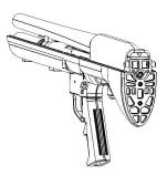
After your shotgun is installed into the lower shroud look at the rear and the bottom two inserts in the adapter block, should line up with the bottom two holes in the lower shroud.
